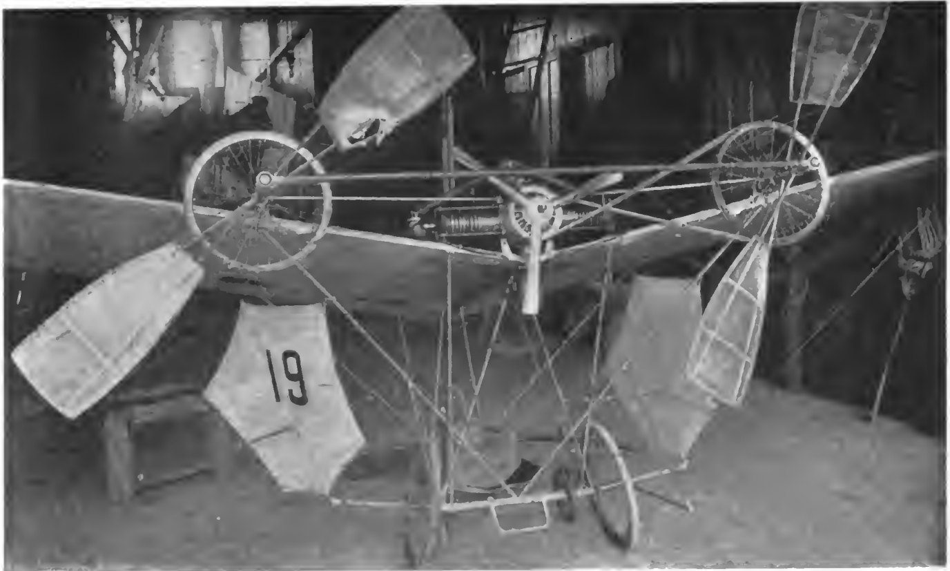
SANTOS-DUMONT'S BUTTERFLY AS IT APPEARS WHEN FITTED WITH TWO ADDITIONAL BELT-DRIVEN PROPELLERS.
